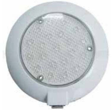
The lamp features 21 super bright LEDs Inbuilt 3 way switch Night light feature All wiring is tinned to reduce the chance of corrosion Very low power consumption of less than 0.10amp Width: 150mm Height: 35mm
