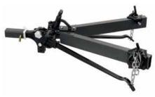
The 800lb kit relies on heavier gauge spring bars than the 600lb to handle heavier trailers. As the name implies, the 800lb kit is designed to work with trailers that have a ball weight between 275kg and 365kg. 800lb - 0818
