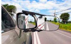
These towing mirrors fit over the existing side mirror to provide added vision while towing. They are fully adjustable and do not obstruct your existing mirror.
