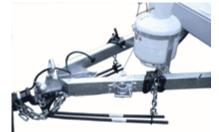
This system has a working range between 80kg and 135kg ball weight and is ideal for small sized caravans.
