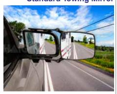
These universal towing mirrors fit over the existing side mirror to provide added vision while towing. They are fully adjustable and do not obstruct your existing mirror. Each
