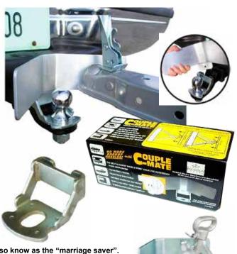
Also know as the "marriage saver". The couplemate fits onto the towbar and will guide your coupling onto the ball. The main body of the couplemate can detatch and be used vertically as a coupling lock so your trailer can be locked onto the ball of the vehicle.
