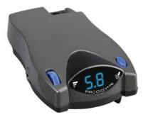
Reverse battery protection for both vehicle and breakaway. Digital display depicts voltage delivery to trailer during braking. No level adjustment necessary. Works proportionally in reverse with the ability to disable when not needed. "Boost" feature gives users the ability to apply more initial trailer braking power when towing heavier trailers. Continual diagnostics check for proper connection. Limited lifetime warranty
