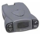
The Tekonsha® P3 features a multi functioning LCD display with the most advanced easy-to-use diagnostics. The P3's convenient features include a dashhugging design, unique easy-to-use clipmounting system, quick disconnect for a safe storage when not in use and the original "boost" feature that allows the driver to increase the initial power delivered to the trailer brakes and capability of switching between an electric brake system or a hydraulic brake system.
