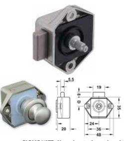
PLEASE NOTE: Size refers to the cupboard wood thickness, not the physical size of the rosette. Both mini and Large suit 16 - 19 mm thickness
