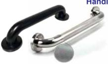
Knurled handle grip section 304 stainless steel 250mm long tube centre to tube centre 32mm tube diameter 1.1mm wall thickness
