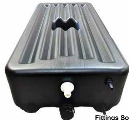
Fittings Sold Separately 25 mm barb inlet 40 mm cap 20 mm plug 3 mm outlet, 13 mm breather Capacity (L): 95 Dimensions (mm): 1170 x 500 x 220
