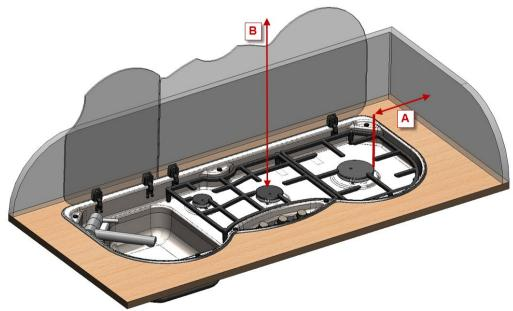
A= 200mm minimum unless protected by a non-combustible heat barrier.
