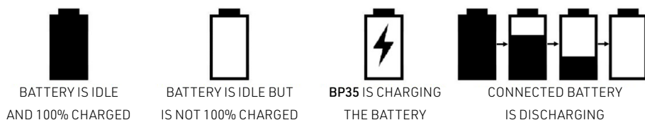
Figure 4: RVView battery status indications
