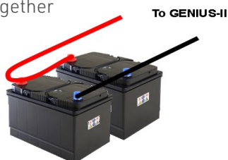
Figure 4: Recommended wiring for connecting batteries in parallel
