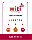
The RESET and PAIR buttons are used to pair WiTi Anti-Theft to a WiTi Wireless Brake Controller or WiTi Wireless Towing Interface. Please follow the instructions contained in those guides for the pairing process.
