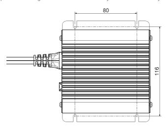
Figure 1: Mounting Dimensions
