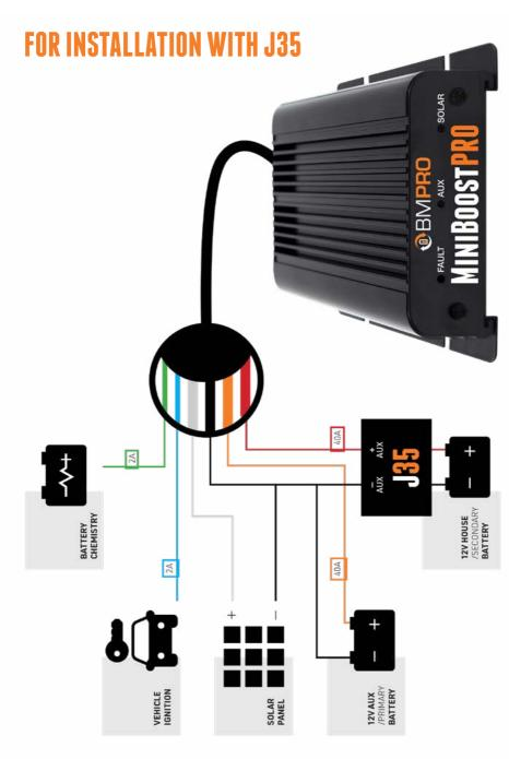
Figure 4: MiniBoostPRO used with the J35
