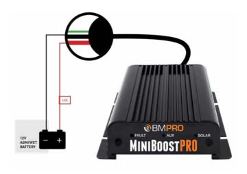
Figure 6: Selecting the 12V AGM/ WET Battery
