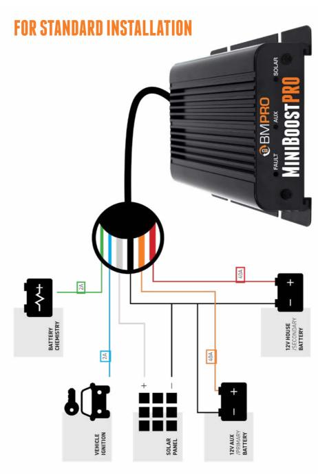
Figure 2: MiniBoostPRO used as a standalone battery charger
