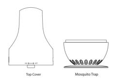
4. To remove the mosquito trap from the top of the unit; rotate the top and bottom pieces as shown above and rotate to the left to pull apart. You can now empty and mosquitoes caught inside; rotate the top and bottom pieces to the right and close tightly.
