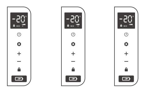
H should be set when the product is connected to car power,and M or L should be set when it is connected to a portable battery or other back-up battery. Because of the different output voltages between vehicles, the battery gear can be set from H to M from M to L if there is a voltage protection code F1 shown on the Panel. The battery gear should be set to H if th product will keep working after turning off the car engine, or the product may drain the battery.
