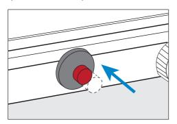
**Note**: If burner does not ignite, return the control knob back to the OFF position, allow the excess gas to disperse then repeat ignition process.
