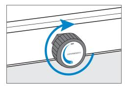
Press the gas control and turn the gas controls full clockwise to the OFF position.
