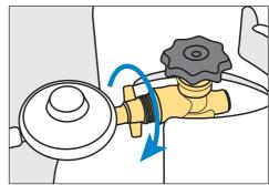
Turn the cylinder gas valve on in an anti-clockwise direction for one full turn and then check the connections for leaks with Companion Gas Leak Detection Spray or soapy water.
