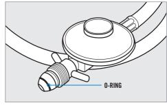
Figure 1: 0-RING seal on the POL regulator.
