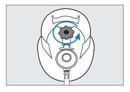
If a leak is detected turn the cylinder gas valve OFF and re-tighten all connections, then retest.
