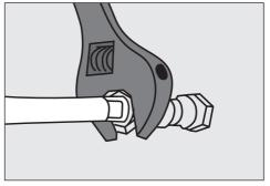
Attach the other end of the hose to the gas cylinder, tightening using the two finger support posts.
