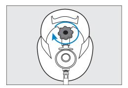
With the flame still operating, turn the valve on the gas cylinder in a clockwise direction until it is OFF. Allow the flame to burn down then extinguish once all remaining gas in the hose has been used.
