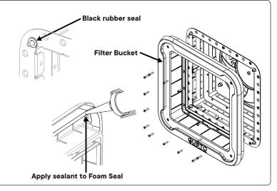
**5.** Insert the Air Filter into the Filter Bucket, ensuring that the pleats are oriented vertically and the pull tabs align horizontally. Insert and fasten the Intake vent by securing 4x captive screws
