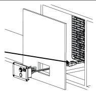
10. Secure the previously cut panel into the cabinet cavity, the method of fastening is up to the installer and will depend on the material of the panel and surrounding cabinet. Ensure that the panel is set back from the front of the cabinet by at least 15mm this will prevent the switch from contacting the cabinet door when closed. Using 4 of the supplied, 22mm long self-tapping screws, fasten the switch panel in place.
